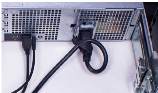
Figure 3. Routing the power cable through the strain relief on a fixed power supply
