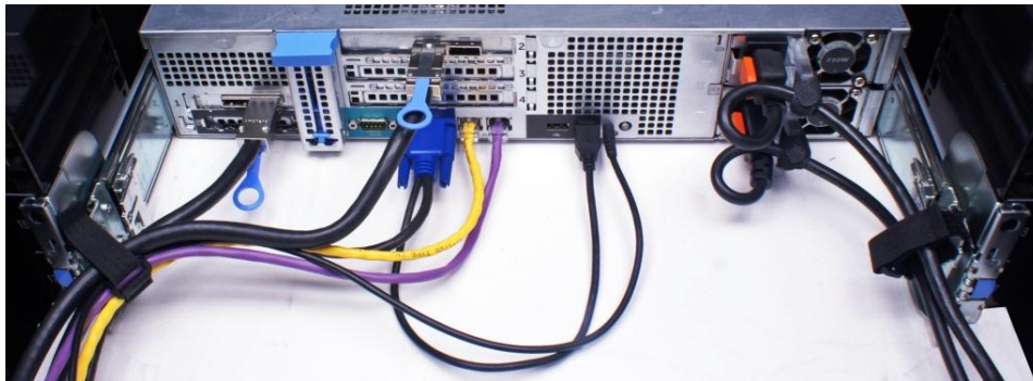
Figure 10. Cable routing on sliding rails without a CMA
