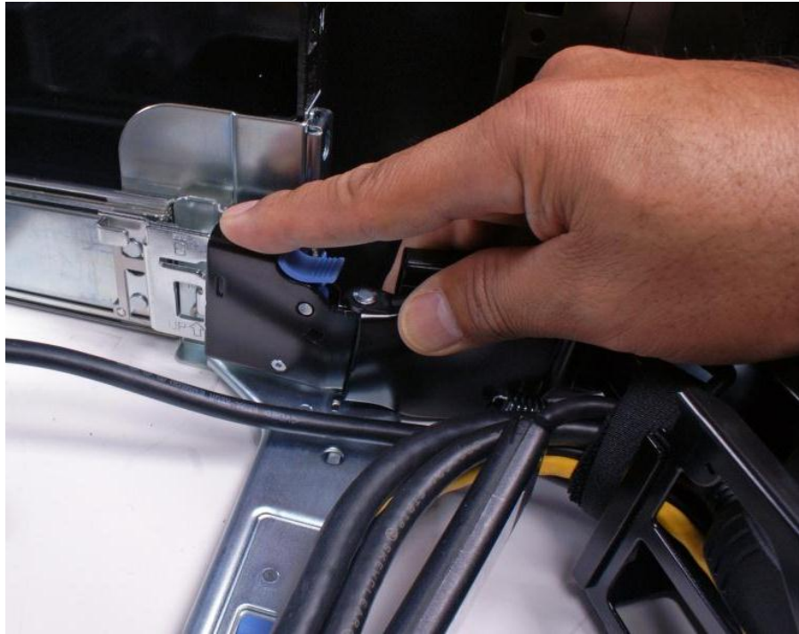
Figure 8. Disconnecting the CMA attachment housings
