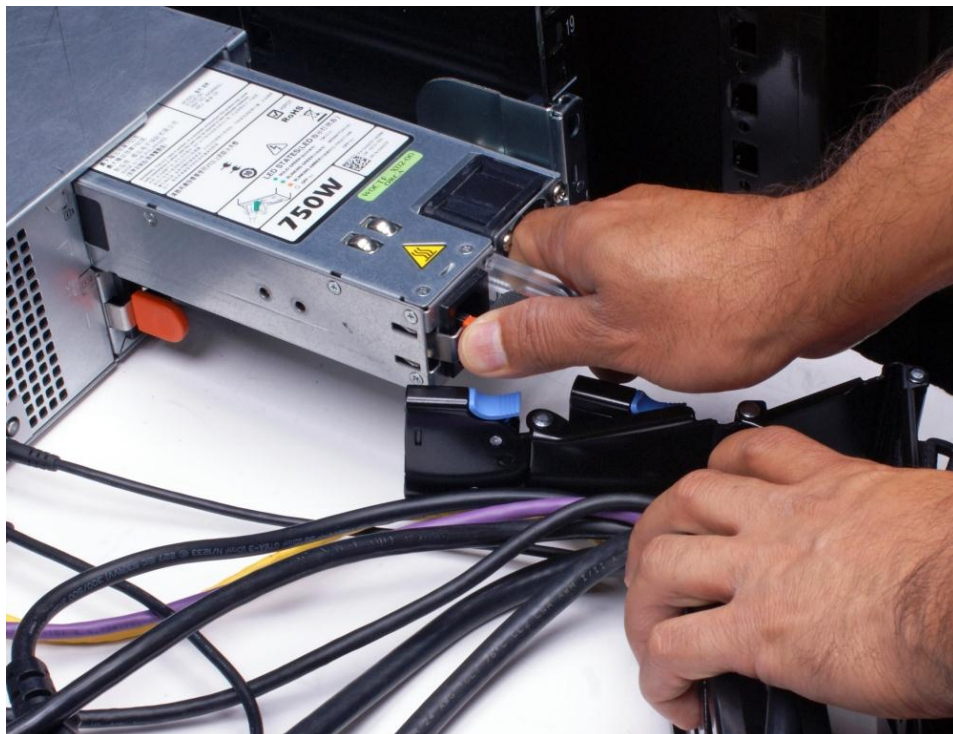
Figure 9. Replacing a hot swap power supply
