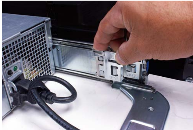
Figure 4. Attaching the inner CMA attachment bracket
